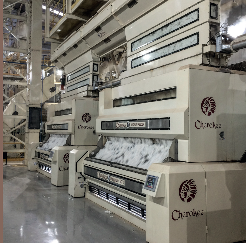
Raw cotton is ginned to separate seeds from lint, then it gets pressed into bales.
